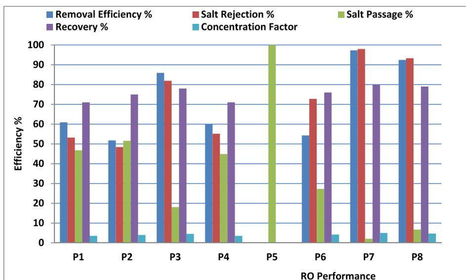
Fig. 11. Reverse osmosis performance in treatment plants (P1, P2, P3, P4, P5, P6, P7 and P8) against contaminates under study.
