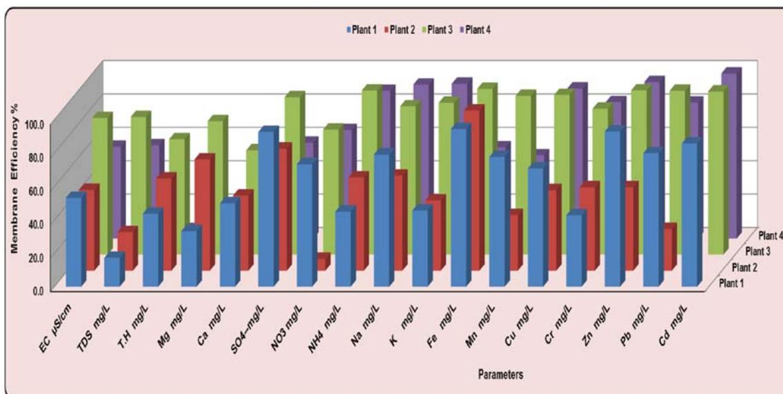
Fig. 9. Membrane efficiency % in reverse osmosis treatment plants (P1, P2, P3, and P4) against contaminates under study.
