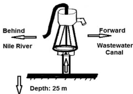
Fig. 5. Drinking pump for underground water.
