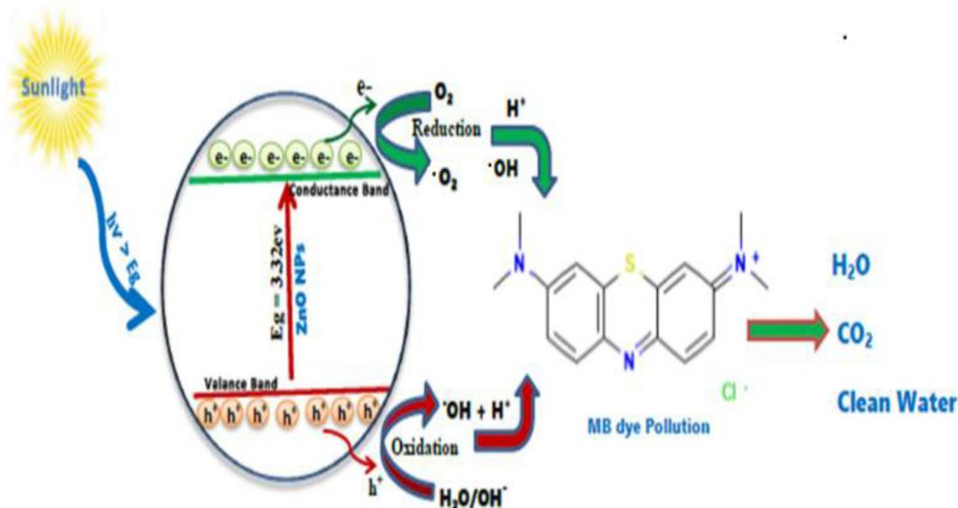
Fig. 14. The suggested process for how zinc oxide nanoparticles photodegrade methylene blue dye.
