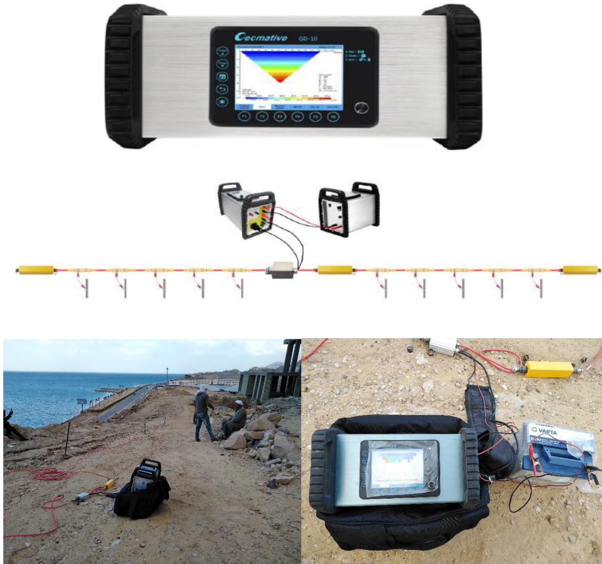
Fig. 4. The geomative GD-10 supreme instrument, field photos for the equipment, and setup of the ERT survey.
