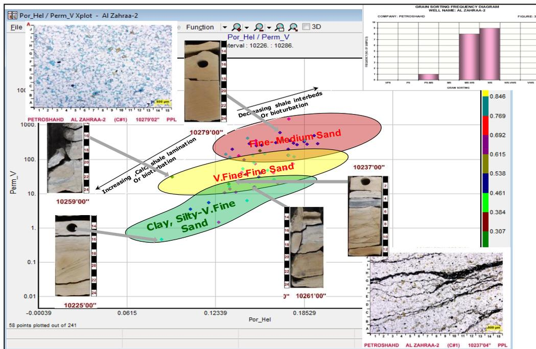
Fig. (6). Core facies classification (porosity vs permeability relative to lithofacies).
