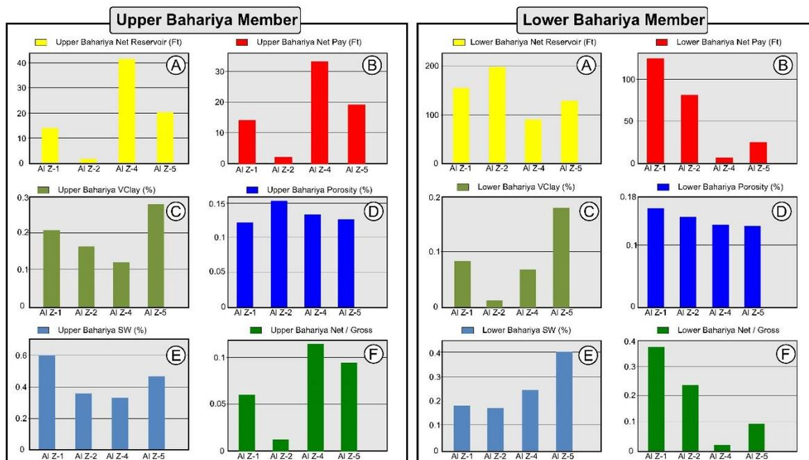
**Fig. (10).** Upper and Lower Bahariya members petrophysical evaluation shows histograms for; (A) net reservoir in feet, (B) net pay in feet, (C) volume of clay in percent, (D) porosity in percent, (E) water saturation percent, and (F) net to gross.
