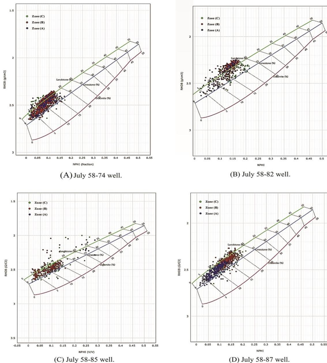
**Figure 5.** Density-neutron cross-plot for different zones of July member reservoir in the available wells ((A) July 58-74well; (B) July 58-82 well; (C) July 58-85 well; and (D) July 58-87 well)).
