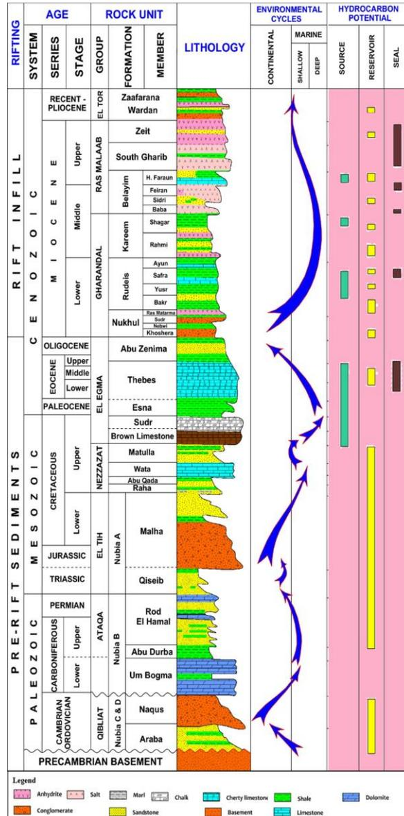
Figure 3. Generalized stratigraphic column of the July oilfield [3].
