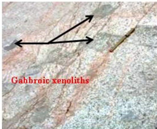
Fig. (2). Gabbroic xenoliths are enclaved by the older granites of Wadi Steih environ.
