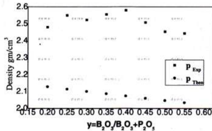
Fig (2) The variation of both the theoretical and Experimental density ( $\rho$ ) as a function of  $y$ .
