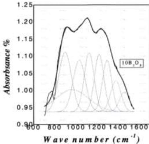
Fig (5) An example of the deconvolution of one of the studied glass sample
