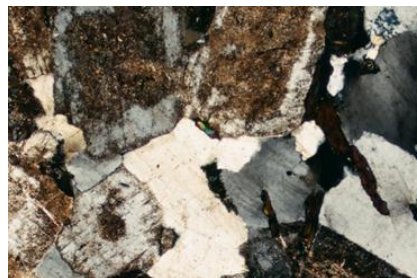
Fig. (15): Photomicrography showing graphic and micrographic texture iron oxides fills most of cracks on the plagioclase and quartz. C.N., X= 40
