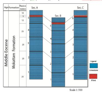
Fig. (21): Measured columnar lithic log of Middle Eocene (Mokattam Formation) recorded at Gebel Kahylia limestone quarry.
