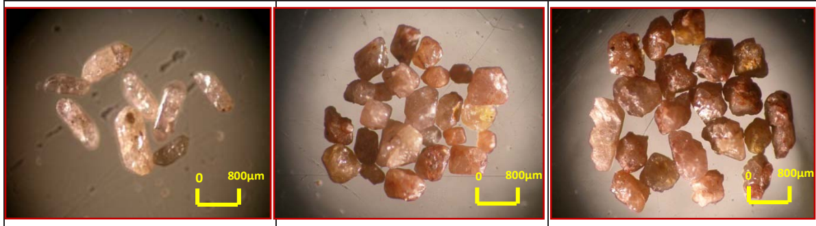
Fig. 15: Photomicrograph of studied zircon showing; -a- Elongated zircon grains of igneous type. b-Zircon grains of mud type. c- Tectonized type (anhedral zircon)
