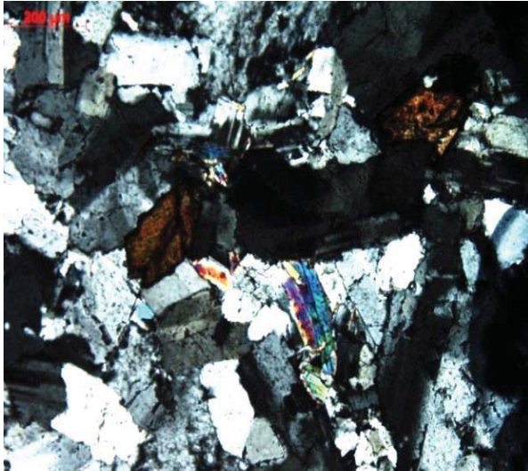
Fig. (23): Photograph showing subhedral albite crystal with anhedral crystals of quartz and muscovite. C. Nin Abu Dabab area
