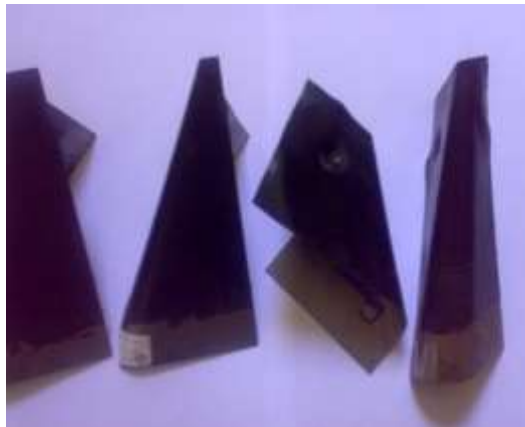
Figure (7): Bending test results for PMA 10 at different NCO/OH ratios
