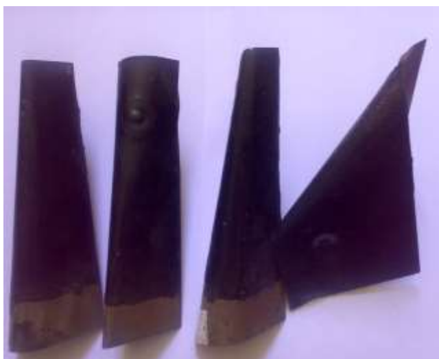
Figure (10): Bending test results for PMA 25 at different NCO/OH ratios
