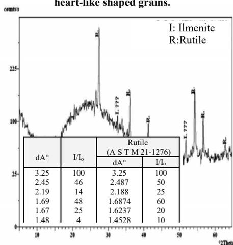
Fig. (13): X-ray diffractograph (XRD) of the black rutile in the non-magnetic fraction II with its ASTM reference values.
