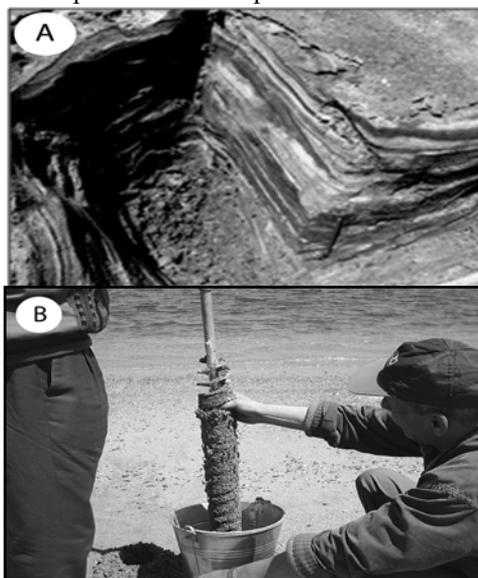
Fig.5: A – Internal structure of Ras Baghdady beach showing regular laminae of heavy minerals (black) alternating with low heavy minerals content (light colored). B – Photograph shows hand auger used for sampling.
