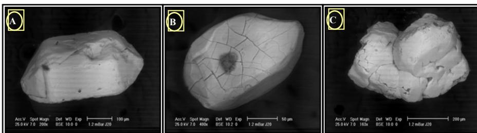
Fig. (22): Back scattered electron (BSE) images show; (A) twinned zircon crystal; (B) zircon grain with fractures radiated from central inclusion; and (C) composite grain of zircon aggregates.
