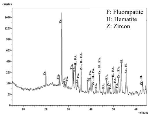
Fig. (23): X-ray diffractograph (XRD) of colorless zircon in the non-magnetic fraction with ASTM reference values.
