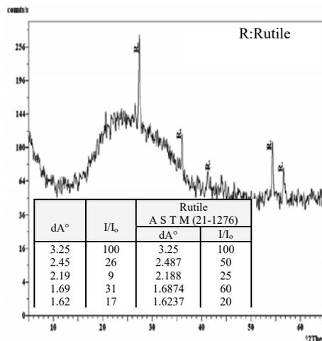
Fig. (14): X-ray diffractograph (XRD) of the reddish brown rutile in the non-magnetic fraction with its ASTM reference values.
