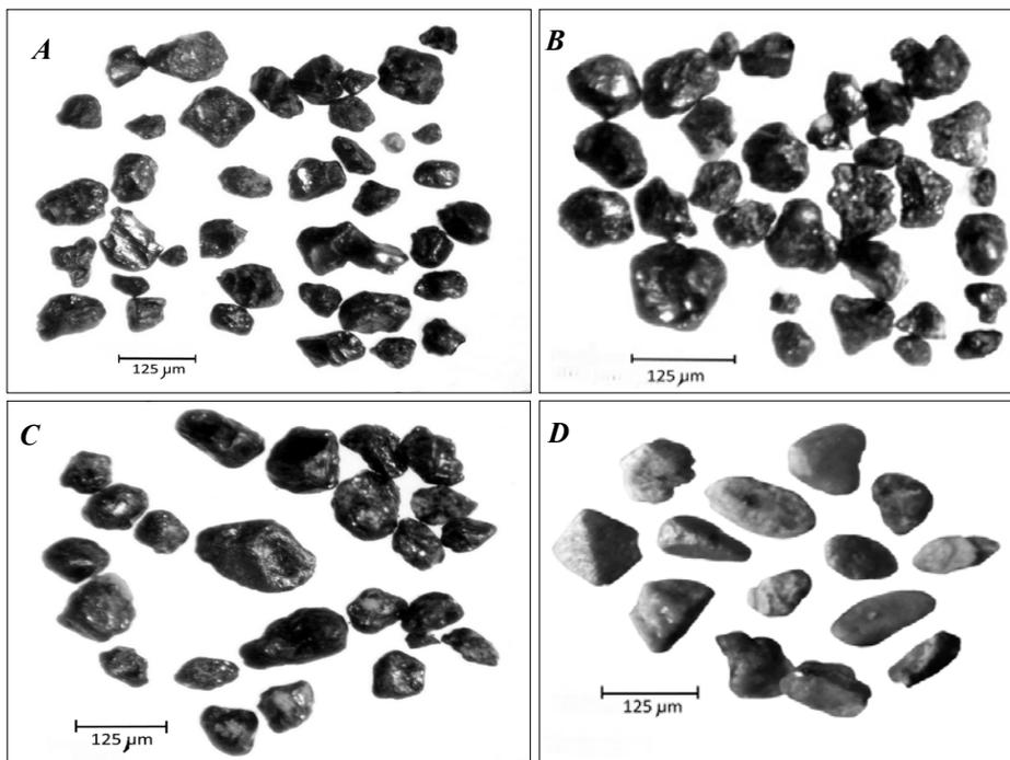
**Fig. (8):** (A) Photomicrographs show;(A) Ilmenite class-I separated at 0.15 amp.; (B) Ilmenite class-II separated at 0.3 amp.; (C) Ilmenite class-III separated at 0.45 amp.; (D) Leucoxenated ilmenite grain separated from the beach sand of Ras Baghdady area, Red Sea coast, Egypt.
