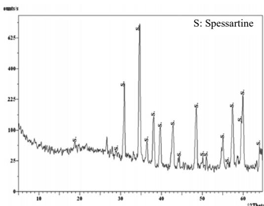
Fig. (20): X-ray diffractograph (XRD) of spessartine garnet with ASTM reference values.
