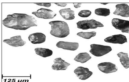
Fig. (19): Photomicrograph shows pink garnet in the magnetic fraction separated at 0.6 amp.
