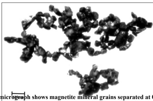
Fig. (15): Photomicrograph shows magnetite mineral grains separated at 0.08 amp.
