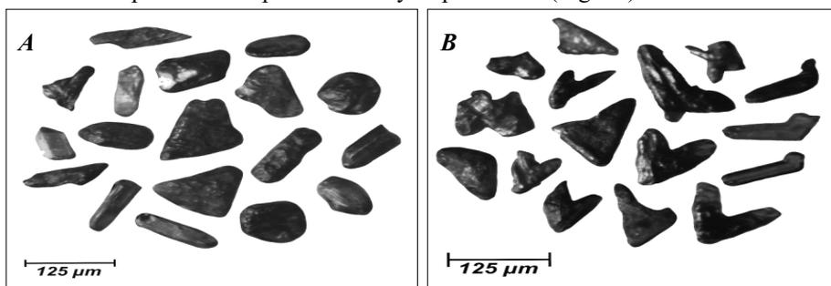
Fig. (12): Photomicrographs showing black and reddish brown varieties of rutile crystals in the non-magnetic fraction separated at 2.0 amp.; (A) elongated, ovate, triangular and tablet-like shaped grains depicting a thick black halo; (B) irregular, elbow twinning (at right) and heart-like shaped grains.
