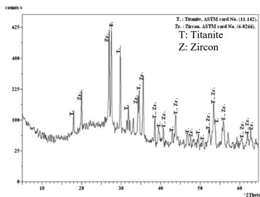
Fig. (24): X-ray diffractograph (XRD) of colored zircon in the non-magnetic fraction with ASTM reference values.
