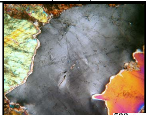
Fig.17: Photomicrograph showing quartz with undulatory extinction and muscovite high order of interference colors (CN).
