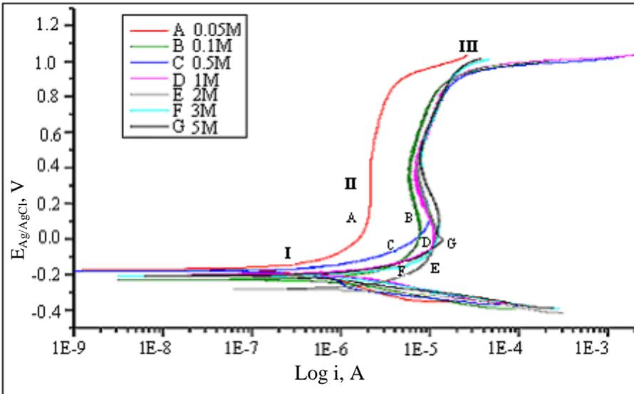
Figure (7): Anodic and cathodic polarization curves of electrode type (II) in (0.05 – 5M) phosphoric acid solutions.
