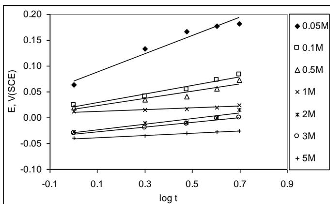
Figure (5): Potential/ $\log t$  relations of electrode II in different concentrations of  $H_3PO_4$  solutions.
